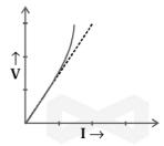
In graph, dotted line part shows that Ohm's law is obeyed, where as continuous curve of the graph shows that Ohm's law is not obeyed.
